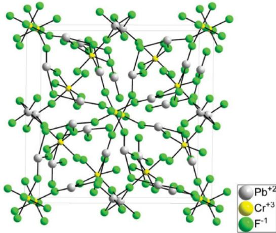
FIG. 1. (Color online) Crystal structure of  $\text{Pb}_5\text{Cr}_3\text{F}_{19}$  (Ref. 5).
