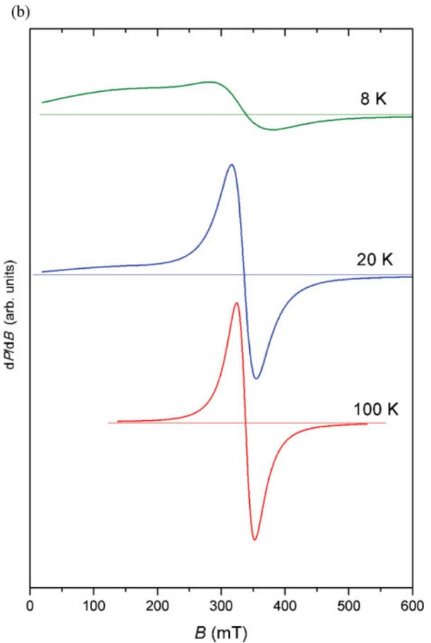
FIG. 2. (Color online) (a) High-temperature X-band EPR spectra of  $\text{Pb}_5\text{Cr}_3\text{F}_{19}$  and (b) low-temperature X-band EPR spectra. The horizontal “zero amplitude line” in (b) helps us see the EPR line asymmetry and the appearance of a new broad line below 20 K.
