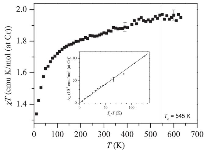
FIG. 9. Temperature dependence of  $\chi \cdot T$  as obtained from ZFC SQUID magnetic susceptibility data of  $\text{Pb}_5\text{Cr}_3\text{F}_{19}$  at  $H = 100$  Oe. The inset shows  $\Delta\chi$  versus  $(T_c - T)$ .
