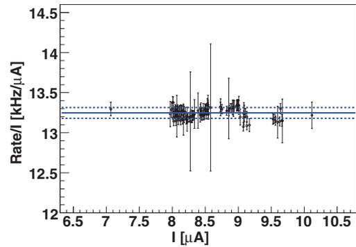
FIG. 6. (Color online) The singles rate in Spectrometer A divided by the beam current for all the  $Q^2 = 0.060$  (GeV/c)<sup>2</sup> runs in the April beam time period. The uncertainties shown are statistical only. The lines show the average and RMS deviation of all the data points. Most of the data are within the uncertainties. Even over a range of 3  $\mu$ A, there is no large target boiling effect.
