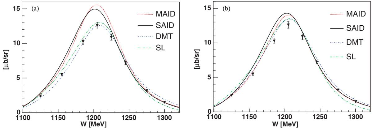
FIG. 11. (Color online) Parallel cross section for the  $p(\bar{e}, e' p)\pi^0$  reaction at  $Q^2 = 0.060$  (GeV/c) $^2$  before (a) and after (b) three resonant parameter fit. Model curves are the same as in Fig. 8. The smaller error bars are the statistical uncertainty and the larger error bars include the systematic uncertainty added in quadrature.
