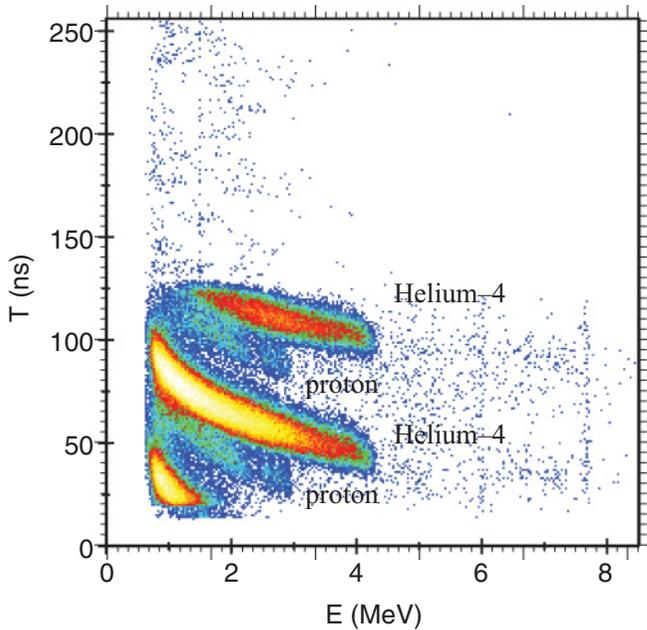
FIG. 1. (Color online) Energy vs time-of-flight spectrum, for all strips of the LEDA array, showing the identification of  $\alpha$  particles and protons. The various particle types are labeled.
