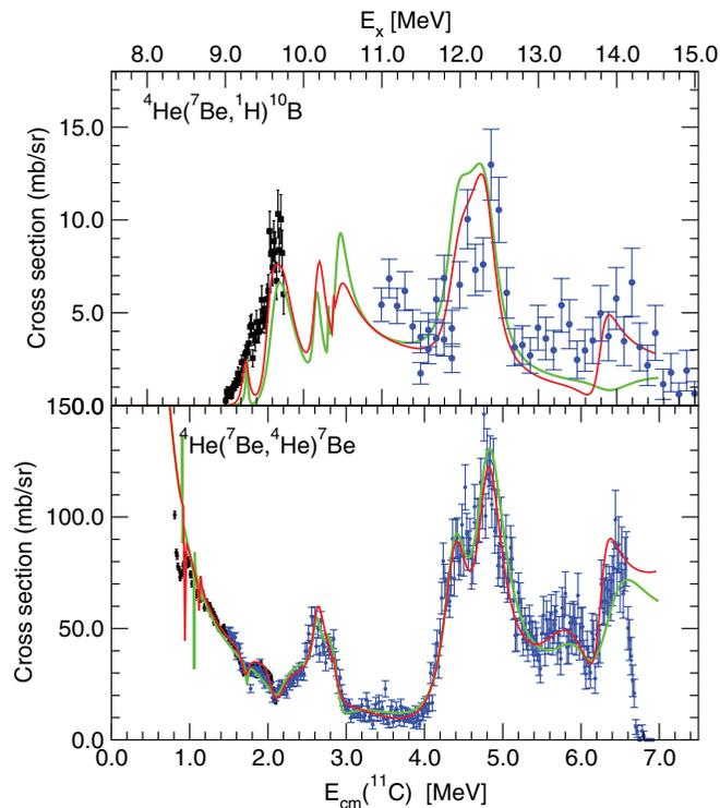
FIG. 3. (Color online) Measured cross sections for the  $^4\text{He}(^7\text{Be}, p)^{10}\text{B}$  (top) and  $^4\text{He}(^7\text{Be}, \alpha)^7\text{Be}$  (bottom) reactions. The red lines show the  $R$ -matrix fit to the data with  $R_0 = 1.4$  fm. Blue data points indicate the high-energy data measured at ORNL and the black data points are the data from LLN. The error bars indicate statistical errors only. The green line shows the  $R$ -matrix fit with  $R_0 = 1.3$  fm.
