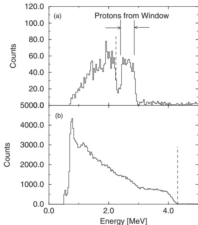
FIG. 2. (a) Proton and (b)  $\alpha$ -particle laboratory energy spectra from the  $E(^7\text{Be}) = 7.1$ -MeV data. The vertical dashed lines indicate the maximum energy protons and  $\alpha$  particles expected from the resonant scattering reactions. In part (a) the region of the spectrum corresponding to protons knocked out of the Mylar window foil is indicated.
