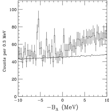
FIG. 3. Binding energy spectrum obtained by the  ${}^7\text{Li}(e, e'K^+){}^7_\Lambda\text{He}$  reaction. The line shows the accidental background estimated by the mixed events analysis method. The events in the unbound region ( $-B_\Lambda > 0$ ) originate from quasi-free  $\Lambda$  production.
