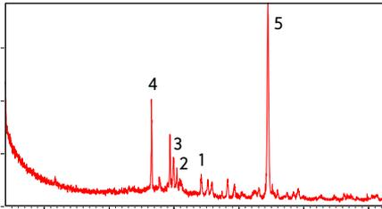
Figure 5. Synthetic minerals: alabandite (1), akermanite (2), clinopyroxene (3), high-temperature quartz (4) and ferosilicomanganese (5) identified by the X-ray diffraction
