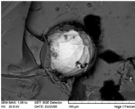
Figure 6. Ferosilicomanganese nodule  $\phi$  60  $\mu\text{m}$  in the glassy slag base, recorded using scanning electron microscope.
