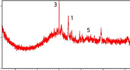
Figure 4. Sample rich in silicomanganese glass which causes increase in the base line. The presence of alabandite (1), clinopyroxene (3) and ferosilicomanganese (5) can be seen on the diffractogramme.
