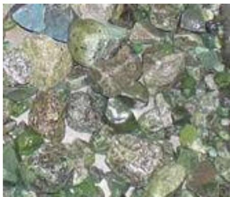
Figure 1. Coarse aggregate of SiMn slag
