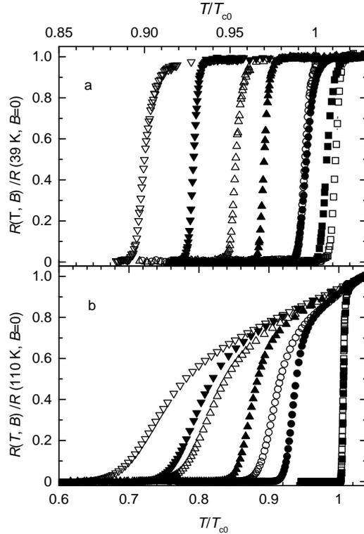
Fig. 1. Temperature variation of the normalized electrical resistance for: a) MgB<sub>2</sub> undoped tape (empty symbols) and tape doped with 5 wt% Si (full) in magnetic fields  $B = 0$  (□), 0.1 (○), 0.4 (△) and 0.9 T (▽), b) control Bi2223/Ag tape (empty) and Bi2223/Ag tape with  $B_\phi = 0.54$  T (Table 1, full symbols) in  $B = 0$  (□), 0.1 (○), 0.4 (△) and 0.95 T (▽).
