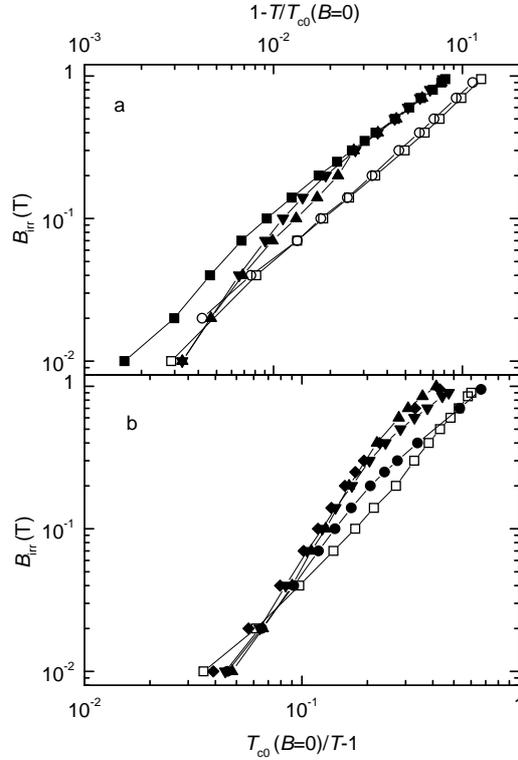
Fig. 2. Temperature dependence of the irreversibility field  $B_{\text{irr}}$  in appropriate temperature scales for a) MgB<sub>2</sub> samples: undoped ( $\square$ ) and Si-doped ( $\blacksquare$ ) wire and undoped ( $\circ$ ), 5 wt% ( $\blacktriangle$ ) and 10 wt% Si-doped tape ( $\blacktriangledown$ ), and b) Bi2223/Ag tapes: undoped ( $\square$ ),  $B_{\phi} = 0.21$  ( $\bullet$ ),  $0.37$  ( $\blacktriangle$ ),  $0.39$  ( $\blacktriangledown$ ) and  $0.54$  T ( $\blacklozenge$ ).
