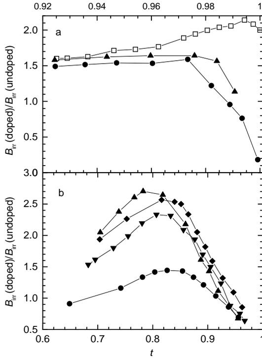
Fig. 3. The ratio  $B_{\text{irr}}(\text{doped})/B_{\text{irr}}(\text{undoped})$  vs. reduced temperature  $t = T/T_{c0}$  for a)  $\text{MgB}_2$  5 wt% Si-doped wire ( $\square$ ) and tapes with  $c = 5$  wt% Si ( $\bullet$ ) and 10 wt% ( $\blacktriangle$ ), and b) Bi2223/Ag tapes with  $B_\phi = 0.21$  ( $\bullet$ ), 0.37 ( $\blacktriangle$ ), 0.39 ( $\blacktriangledown$ ) and 0.54 T ( $\blacklozenge$ ).
