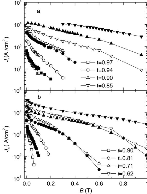
Fig. 4. Field variation of critical current density  $J_c$  at reduced temperatures denoted on plot for the: a)  $\text{MgB}_2$  undoped wire (empty) and 10 wt% Si-doped tape (full symbols) and b)  $\text{Bi2223/Ag}$  undoped tape (empty) and tape with  $B_\phi = 0.54$  T (full symbols).
